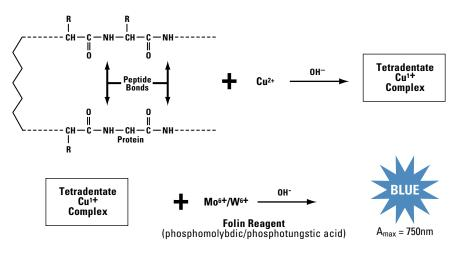
Figure 1. Reaction schematic for the Modified Lowry Protein Assay.
