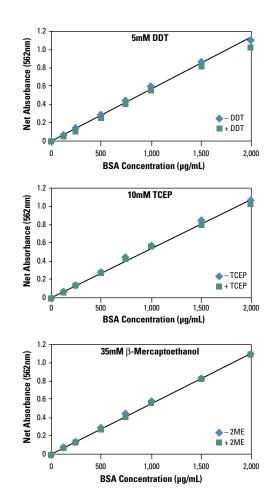
Figure 1. Thermo Scientific Pierce BCA Protein Assay – Reducing Agent Compatible produces a linear standard curve in the presence of reducing agents. Color response curves for BSA after treatment with Reducing Agent Compatible Reagent in the presence and absence of 5mM DTT, 35mM  $\beta$ -mercaptoethanol and 10mM TCEP.
