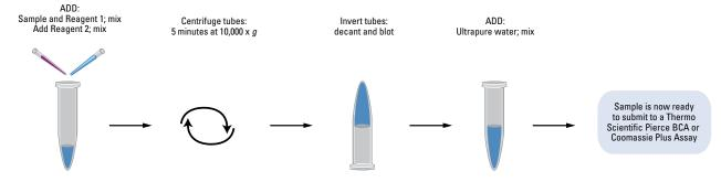
Thermo Scientific Compat-Able Protein Assay protocol. Make almost any protein sample compatible with the Thermo Scientific Pierce BCA or Coomassie Plus (Bradford) Assays in four simple steps.
