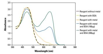
Figure 1. The absorption maximum of the reagent-metal complex shifts proportionally upon binding to BSA. The absorption spectra were recorded for the Thermo Scientific Pierce 660nm Protein Assay Reagent from 340 to 800nm using a Varian Cary<sup>®</sup> Spectrophotometer. The assay reagent is a proprietary dye-metal complex that binds to protein in acidic conditions, which shifts the dye's absorption maximum.
