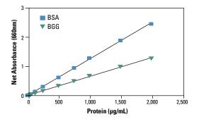
Figure 2. Typical color response curves using the test tube procedure. The linear detection ranges are 25-2,000µg/mL for bovine serum albumin (BSA) and 50-2,000µg/mL for bovine gamma globulin (BGG). The average absorbance for the blank replicates (control) was subtracted from the absorbance for individual standard replicates.
