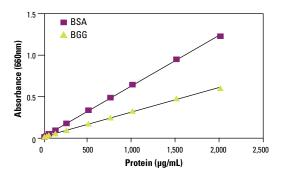
Figure 3. Typical color response curves using the microplate procedure. The linear detection range is  $50-2,000\mu$ g/mL for bovine serum albumin (BSA) and bovine gamma globulin (BGG). The average absorbance for the blank replicates (control) was subtracted from the absorbance for individual standard replicates.
