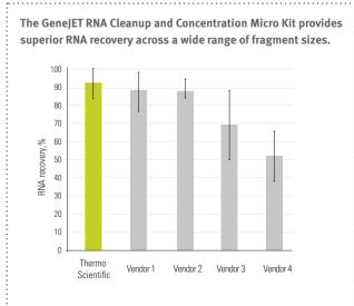
RNA of different length (500 bp, 6000 bp or total RNA) was concentrated using recommended protocol from different vendor kits. The data represents average recovery combining RNA yields for all different RNA lengths. RNA concentration was estimated using a NanoDrop spectrophotometer.
