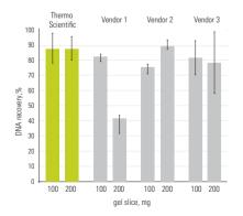
Following gel electrophoresis of 1 µg (900 bp) DNA fragment, gel slices of various size (100 mg and 200 mg) were purified using recommended gel extraction protocols from different vendors kits.
